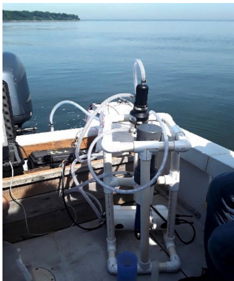
Pump used for measuring water-quality parameters for hydrodynamic study (l) and sensors for bottom-water measurements (r) (photos by Carol DiPaolo, 6/13/24)
